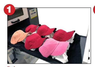
**Step 1:**Pretreat the hats with 15 to 20 grams of pretreat. To aid in an even print you can use a gloved hand or synthetic bristle paint brush to smooth out the pretreat on the cap. If printing CMYK only, this step is not needed.
